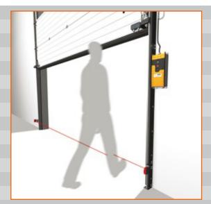
rail. If the beam between the transmitter and the reflector/receiver is broken, a signal is sent to the motor to stop and reverse the movement. While the reflector system is sensitive to dust and moisture, this is not the case for the receiver model.
