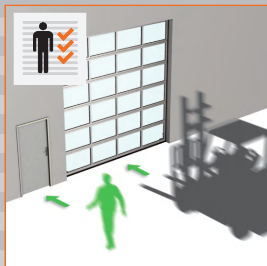
Completely separate doors for pedestrians and goods.
