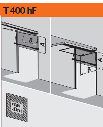
T 400 hF Elevated rail system with low spring axis + steel support profile
