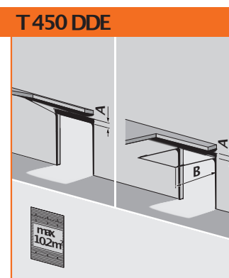
T 450 DDE Normal lift track system with pre-assembled low-mounted spring shaft assembly
