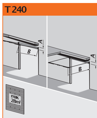
T 240 Low built-in rail system, incorporated cables + steel support profile
