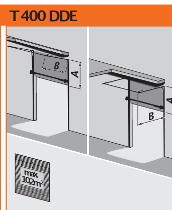
T 400 DDE Springless elevated rail system
